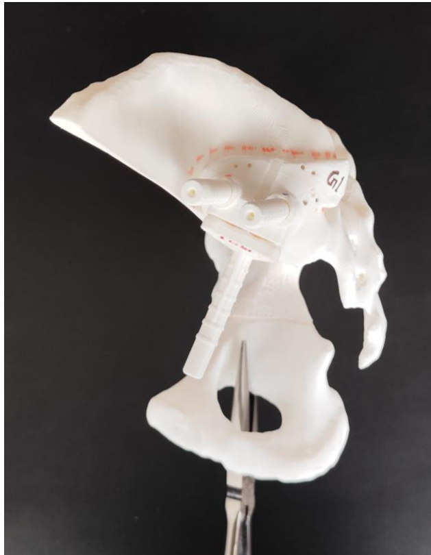
Fitment of guide wire jig assembly onto the resected bone
