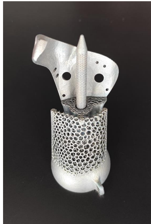
Fitment of dummy implant onto the resected bone surface
