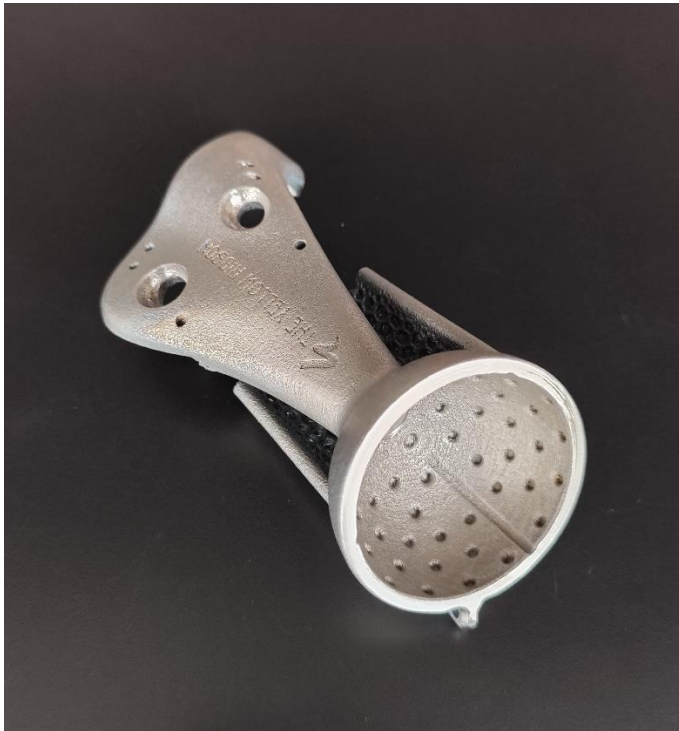
Custom 3D printed Titanium implant
