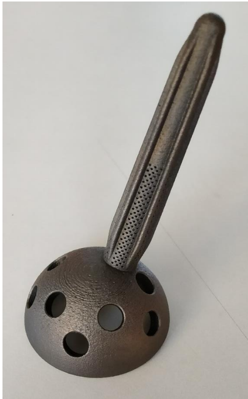
Dummy implant model (top); Actual Implant – Ti64 (bottom)
